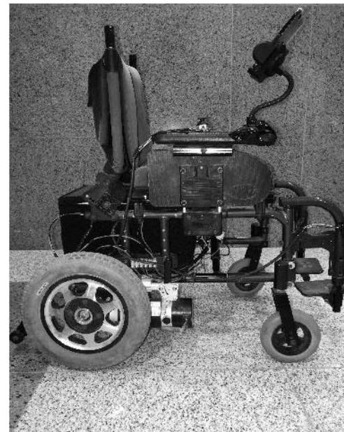
Figure 1. Smart wheelchair with sensors and a mobile phone attached on its armrest
