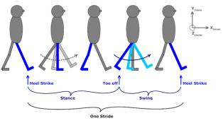
Figure 2: complete gait cycle.
