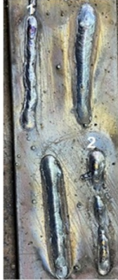
Figure 5. Weld beads resulting from two different welding speeds
